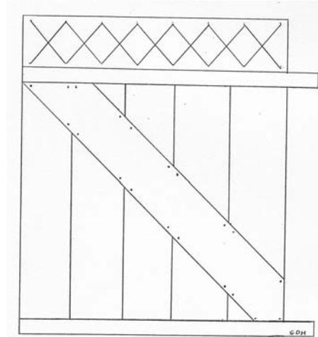
**Above:** Sketch of half door section at near end or southwest wall of Wemple barn. Note scribed Xs on batten on rear face of door.
